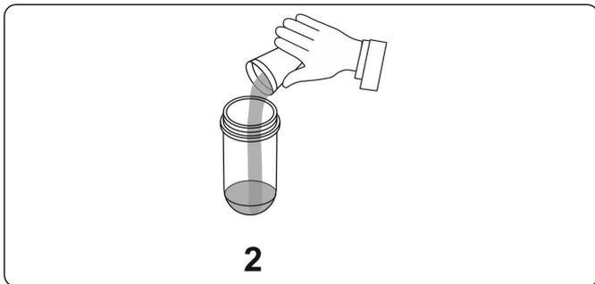
Cut a corner of the 80 gr sealed bag with the Cillit®-55 M-H Universal and pour the whole content into the water of the basin.
