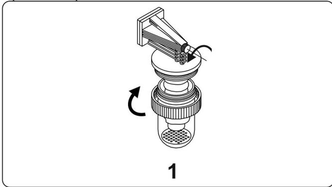
Clean the basin, the bellow and the solubilisation disc with clean water. Pour a glass of water (60 cc) into the basin.
