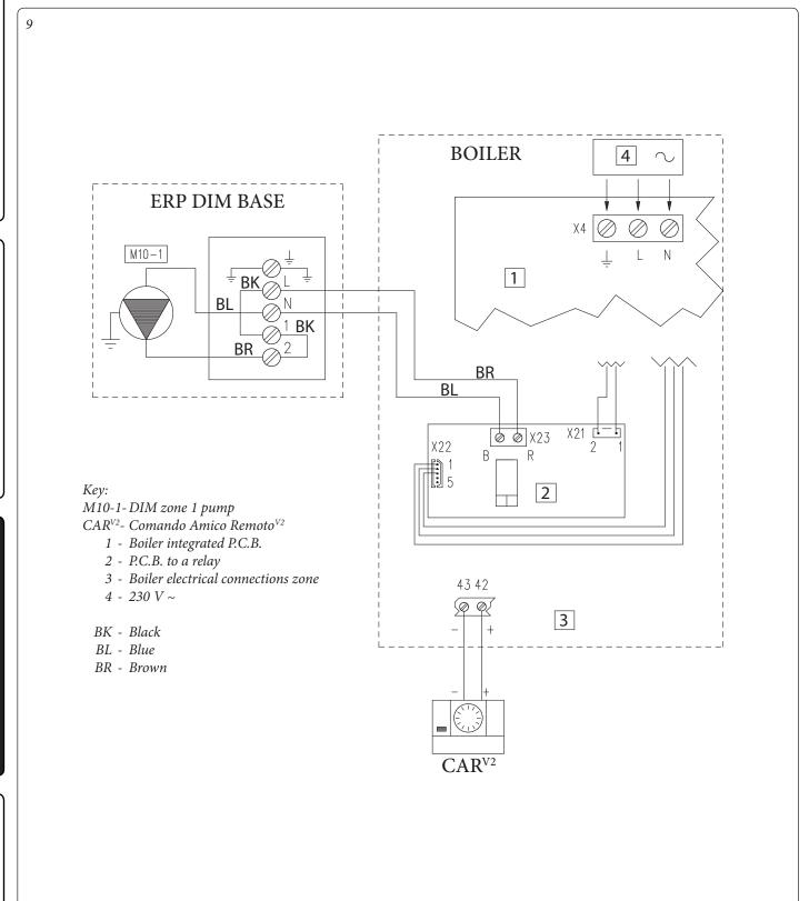
Only use for boilers equipped with the Comando Amico Remoto  $^{\rm v2}$  remote control and the internal 1 relay board. In this case the electrical connection of the CAR $^{\rm v2}$  must be made directly to the boiler as described in the relative instruction book.
