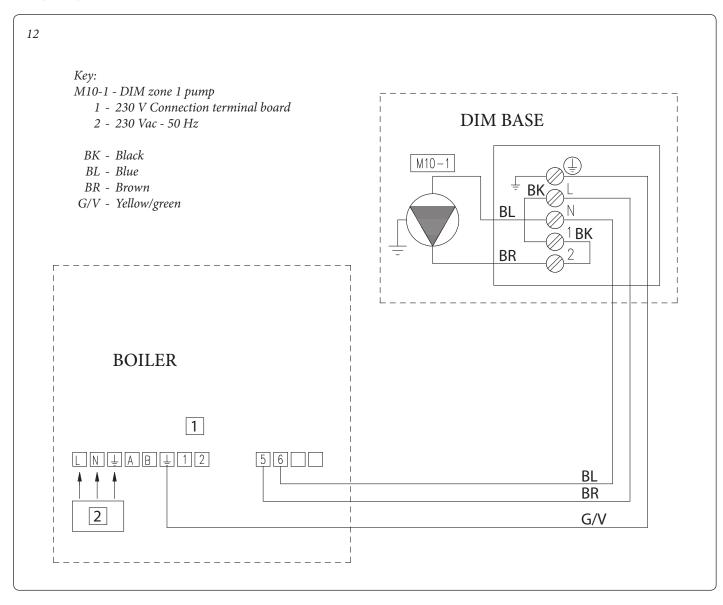
Configuration required on boiler board: Multifunction relay (K70), with P.4 = 6 (central heating mode active).
