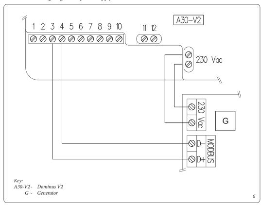
$\textbf{N.B.:} \ for \ connection \ to \ the \ power \ supply \ line \ (230 \ Vac), \ provide \ a \ double-insulated \ electrical \ cable.$
