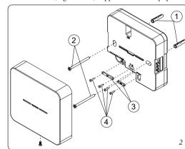
Once the electrical connection has been done, close the Dominus V2 device by fastening its protective cover (Fig. 3 Ref. 1) with the specific screw (Fig. 3 Ref. 2).
